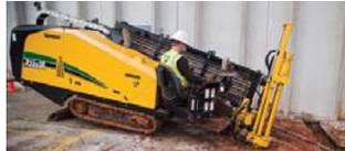
The D23x30 S3 Navigator® horizontal directional drill is one of the quietest drills in the market. With a 100-hp engine, the D23x30 S3 offers speed and power in a short, narrow footprint to help increase productivity when working in compact urban or commercial jobsites.
