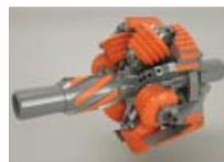
The newly developed Full Face Hole Opener enables the contractor to drill
