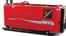
HammerHead HydroBurst 100XT static pipe bursting system – The HydroBurst 100XT static pipe bursting system delivers 98 tons of pulling force for sewer, water and gas line replacement jobs. The streamlined 100XT's production rates are up to twice as fast as its predecessor thanks to the pipe bursting industry's first automated rod spinning assembly and the unique design of its hydraulic cylinders.
