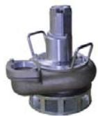
The S4TAL-2 solids handling pump features a cast, machined aluminum volute, stainless steel wear plates and a two vane channel impeller. Delivering output flows to 700 GPM, heads to 100
