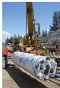
Robbins specializes in small diameter boring equipment, which includes Small Boring Units (SBU-A), Motorized Small Boring Units (SBU-M), Rockheads
