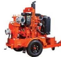
The Godwin Dri-Prime® CD150M pump offers flow rates to 2,290 GPM and has the capability of handling solids up to 3.0" in diameter. The CD150M is able to automatically prime to 28-ft. of suction lift. Automatic or manual starting/stopping is available with mounted control panel or optional wireless remote access.
