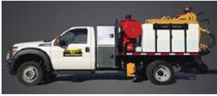
The new HTV (Hydro Truck Vac) PTO (Power Take Off) Truck series has debris tanks ranging from 300 gallon to 1500 gallon in size. The PTO of the truck drives positive displacement vacuum blowers that produce 1,000 to 3,000 CFM. These units are standard with a high pressure water system, full hydraulic rear door, reverse pressure, and the patented "Big Red" filter housing. Air compressors and Hydraulic booms are also available.
