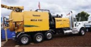
from 1,200 to 3,000 gallons (4,542.5 to 11,356.2 L) and a standard option of 800 gallons (3,028.3 L) of fresh water. It has a 6-inch (15.2 cm) hose width with a 3,200 CFM (91 m<sup>3</sup>/min) blower at 18 inches of mercury. It is powered by a 200-horsepower (149 kW) John Deere Tier 3 engine, and features a 3-stage cyclonic filtration.
